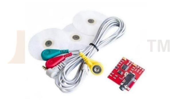
The Advance Technologies EMG Muscle Sensor V3.0 With Cable And Electrodes will measure the filtered and rectified electrical activity of a muscle; outputting 0-Vs Volts depending the amount of activity in the selected muscle, where Vs signifies the voltage of the power source. Power supply voltage: min. +-3.5V.
